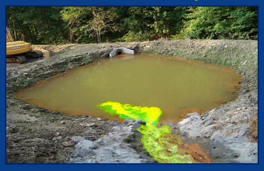
Retention time would not have been much anyway, but due to the specific flow path, it was around 4 minutes. Could you have envisioned that this is how the water would flow? Was there some way to mathematically determine that this would happen? Have you started to catch on to where I am going with this???? Before moving on with solutions for these types of problems, let's just look at a couple more examples.
