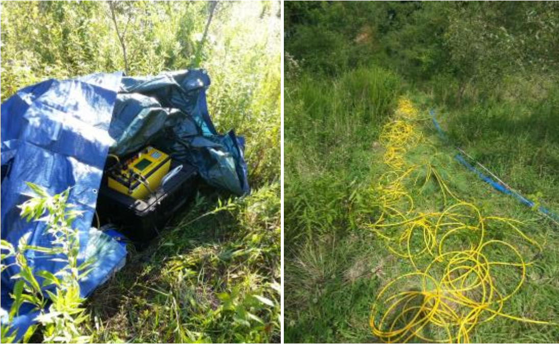
Figure 3. ERI equipment: AGI Earth Imager unit (left) and transect of electrodes connected by electrical cables (right). (Photo credit: Breeyn Greer).
