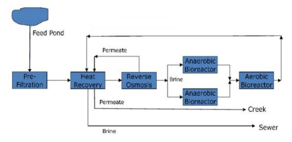
Figure 2 - Process Flow Diagram Active Selenium Bio-treatment at a Western US Metal Mine
