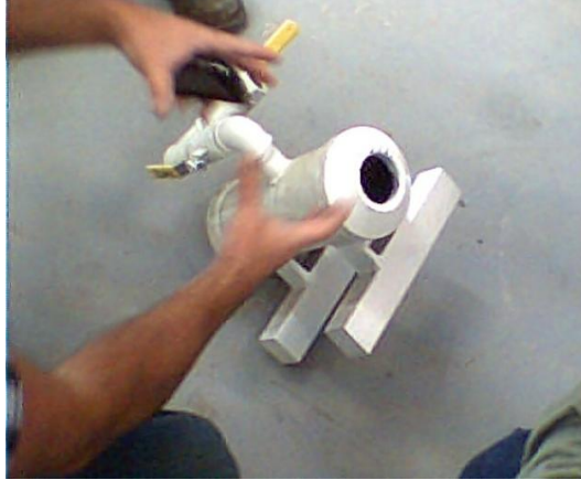
Figure 3. Static mixer used to combine solid and foam components to create pHoam™
