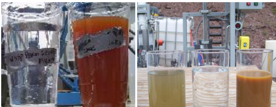
Figure 5: VSEP Permeate and Concentrate
