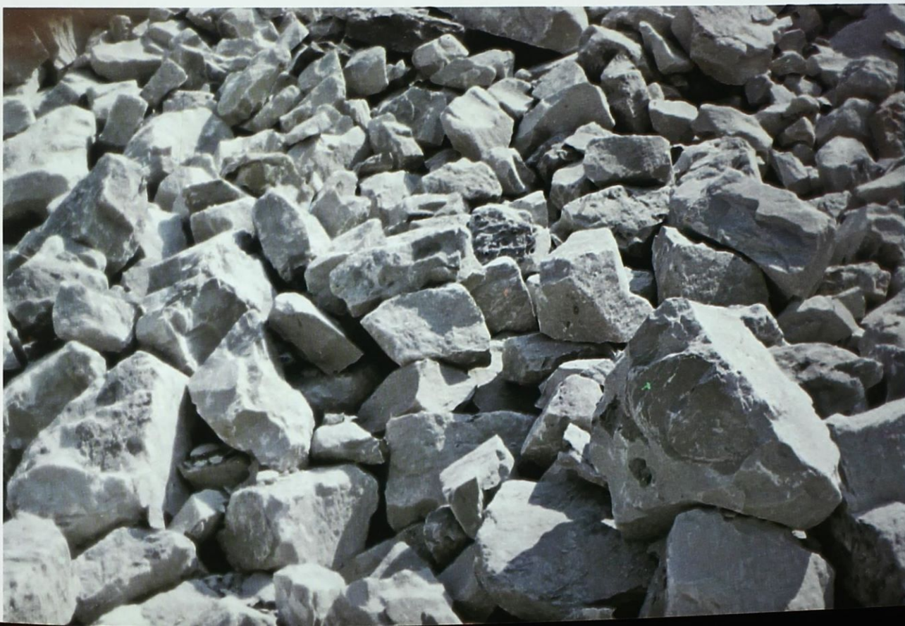
The rock drainage blanket is formed by gravity separation.
