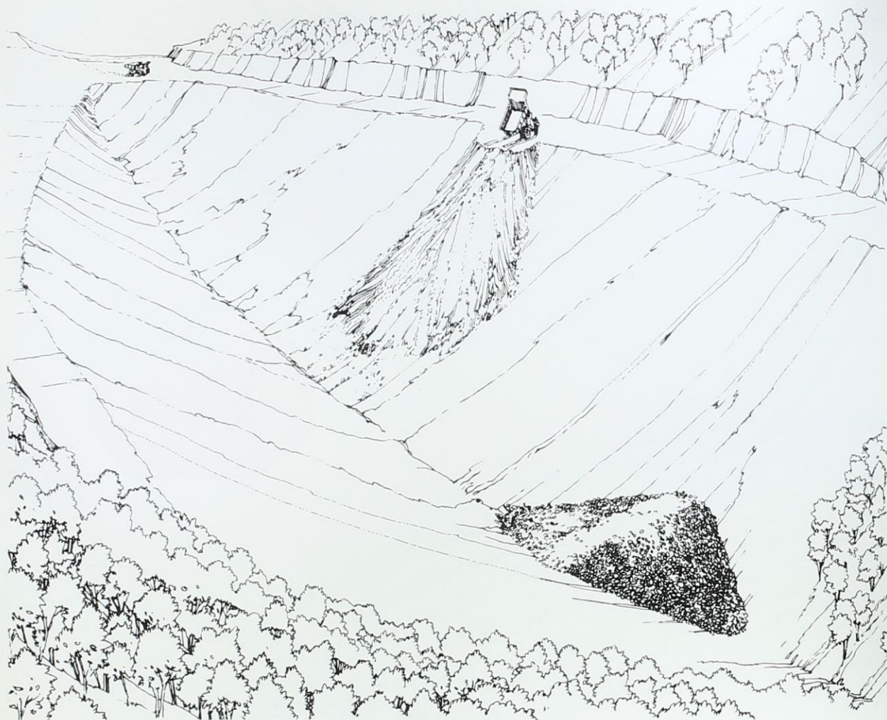
Side Dumping With Physical Support Construction
