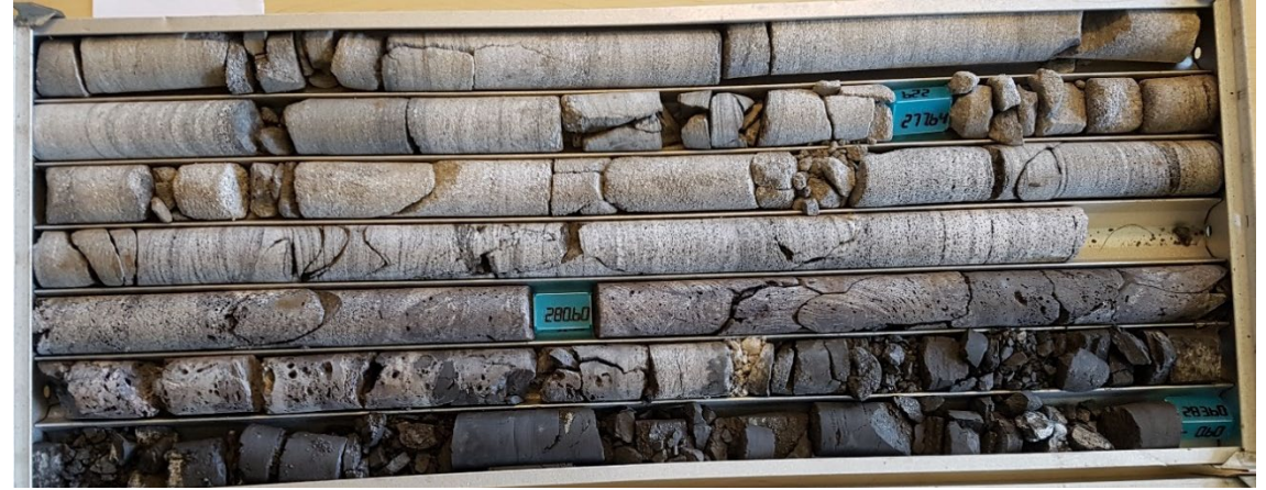
Heat affected sandstone
