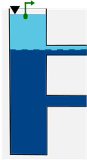
low pumping rate, pump above stratification → stratification breakdown less likely
