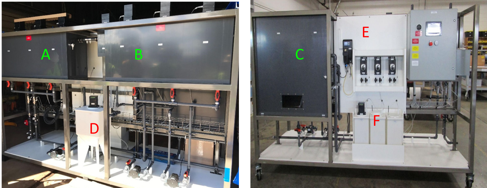
A - Reaction Tank; B - Flocculation Tank; C - Sedimentation Tank; D - Sludge Holding Tank; E- Chemical Dosing Pumps; F - Chemical Storage Tanks
