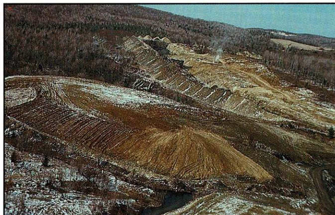
The remining operation at Benbush was 211 acres, daylighted old auger holes from previous surface mining and eliminated old highwalls. Picture taken March, 1983.
