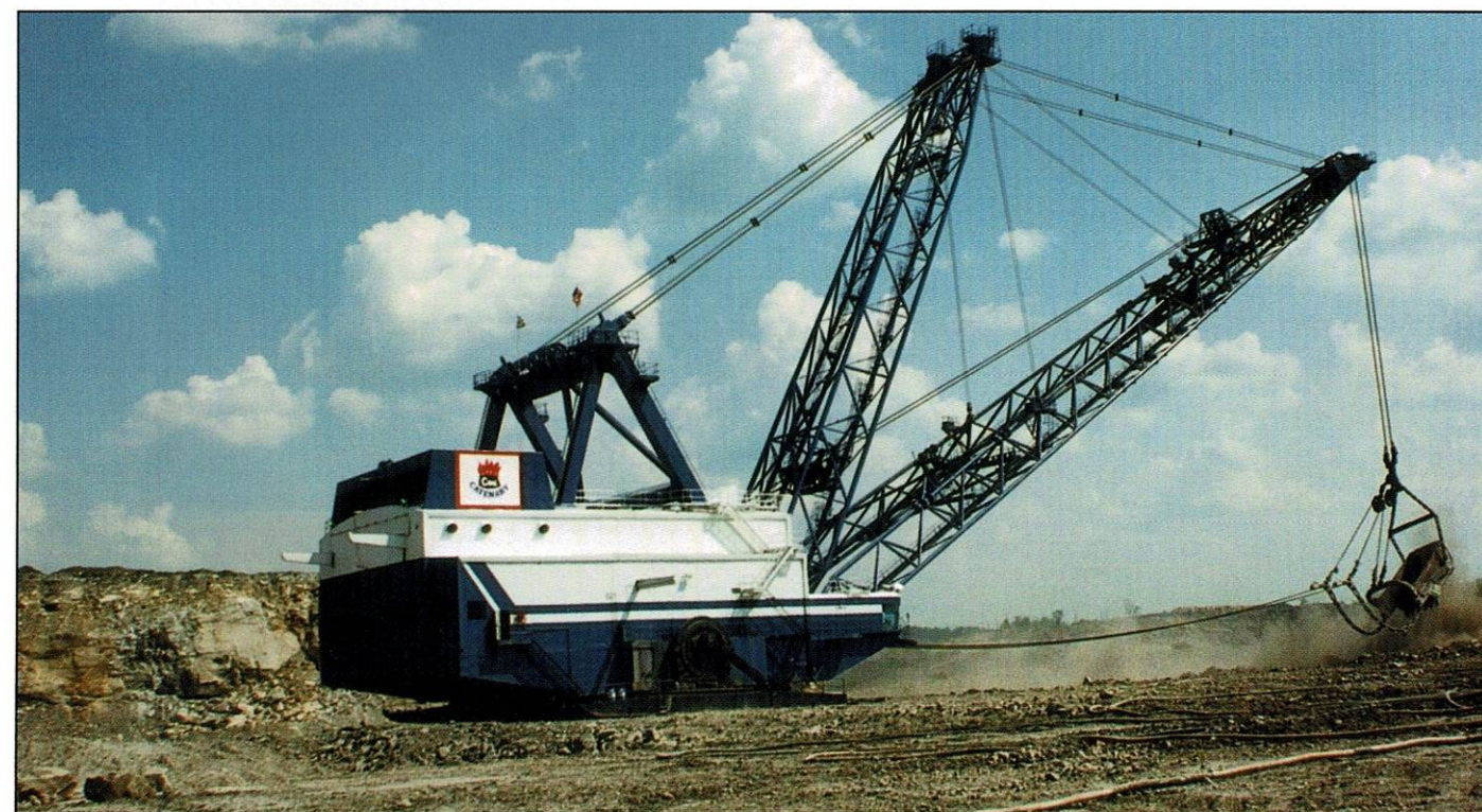
Catenary Coal's 100 yard dragline is now the largest piece of mining equipment in West Virginia.
