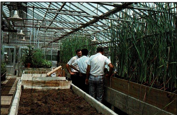
Wetlands have been constructed in greenhouse troughs where temperature and water flows can be controlled. Some of the troughs receive acid mine drainage while others receive rain water at the same rate. With special equipment and procedures, chemical and physical reactions, microbial processes, and plant productivity can be monitored in these wetlands. An understanding of these processes may help us build more efficient wetland systems.
