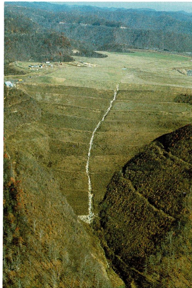
Excess overburden from mountaintop mining operations is routinely placed in valley fills, where the terraced slopes and rock core center control drainage off the mountain and into sediment ponds.
