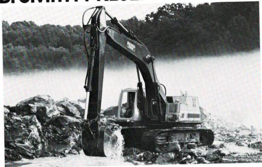
The 325–H, tackles tough jobs requiring a machine with capacities up to  $2\frac{1}{2}$  cu. yds. It has all the superior features which make the B–E 100 Series excavators the preferred back hoes: strong breakout force, high lift capabilities, and rugged construction in boom and handle which eliminates stress buildup...reduces chance of boom and handle failure. You get improved durability and availability in the toughest digging.
