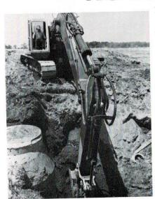
The 325-H reaches far, digs deep, dumps high. Demand/control high pressure hydraulic system automatically adjusts speed and force on any digging cycle for peak productivity.
