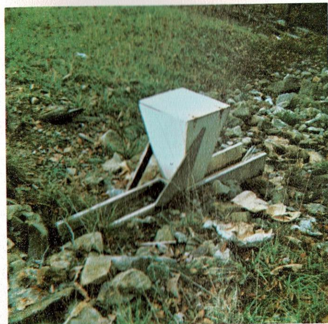
EPA has conducted successful tests on units like this, which employ sodium hydroxide as a neutralizing agent.
