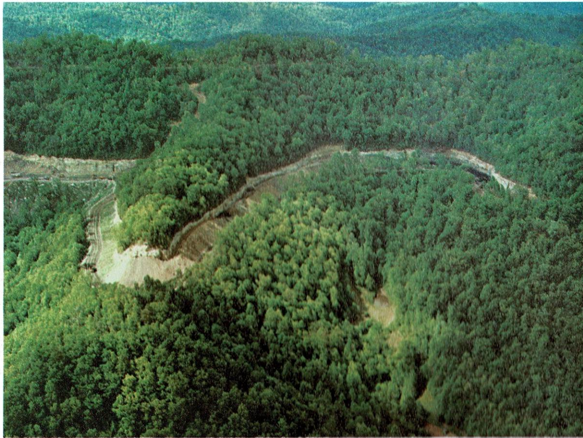
An aerial view of Hobet's Trace Fork job reveals the difference between old and new methods. At the left is an old permit which allowed downslope spoil placement and highwall retention. To the right is a clear illustration of the reduction in disturbed area. Note the sediment control structure to the right of center.
