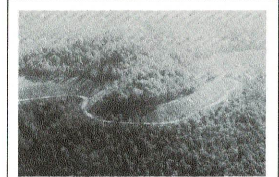
The haulback method reduces the disturbed area by nearly two-thirds when compared with conventional surface mining.
