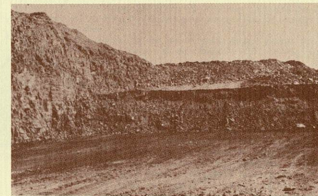
Figure 8: A working block before coal is removed. Ultimate highwall is on the left and the working wall on the right.
