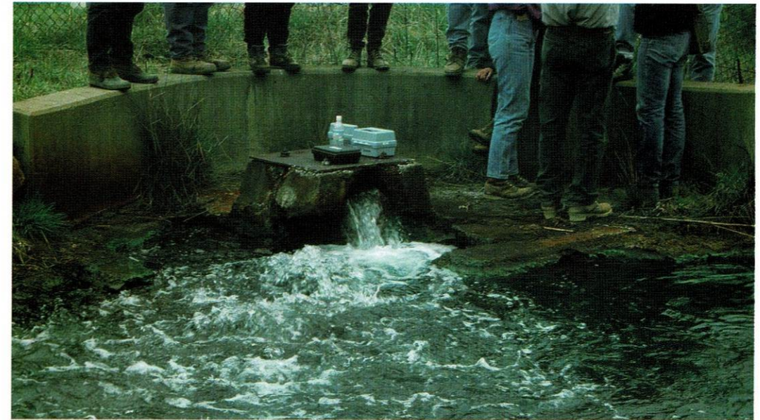
Acid water from an abandoned underground mine is being discharged from this point source into a major stream. For streams like this one that cannot meet the water quality standards, TMDLs will be developed in order to reduce the pollutant load in the stream. A large acid mine drainage chemical plant is being designed to treat the water and reduce the pollutant load to the stream.
