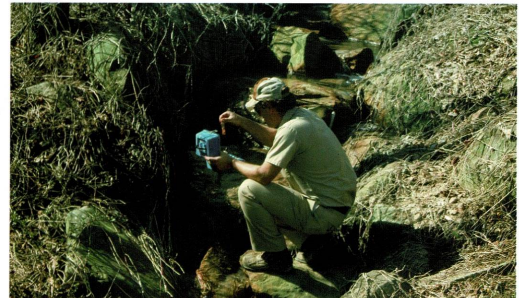
Water samples are routinely taken at water discharge points and analyzed by entities holding NPDES permits. The entity must submit a report each month providing data on water quality for specified effluent limits at the discharge point. Inspectors of the West Virginia Department of Environmental Protection check the quality of water at discharge points to determine whether effluent limits are being met when they visit mine sites.
