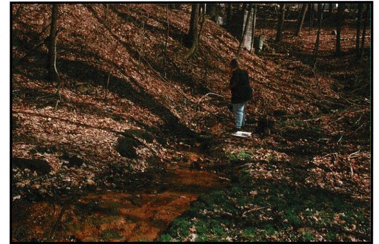
Site 88 is an undisturbed site. The seep emerges from the collapsed portal, creating a large area of Fefloc.
