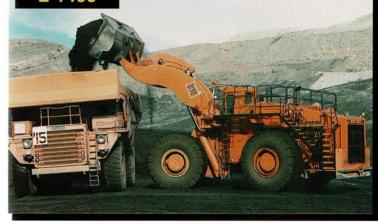
From the development of the first LeTourneau loader in the early 1960s to today's L-1800, LeTourneau has been and continues to be the only loader manufacturer to install electric motors inside the wheels where power is needed most.
