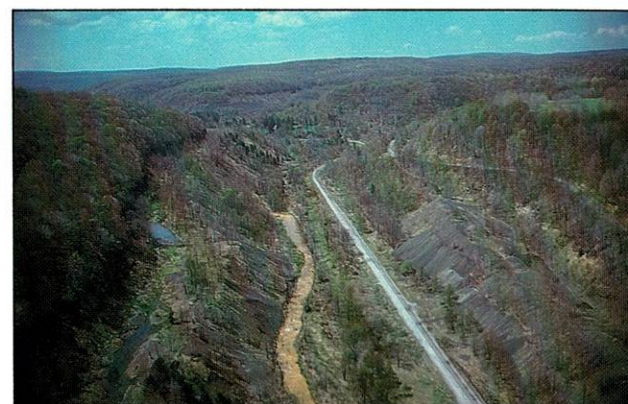
Picture 5. Aerial photograph of the Douglas Highwall AML Project before construction. Highwalls and benches can be observed on the left along with a large refuse pile on the right. The North Fork of the Blackwater River is in the center paralleled by the railroad bed. This picture was taken on May 11, 1992 before construction occurred.
