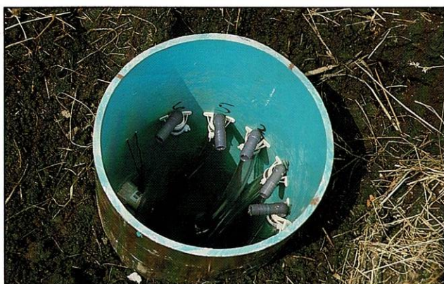
Picture 4. Thirteen sampling tubes were installed in the treatment system. Each tube contains 5 ports from which water and sediment samples can be extracted from 5 different depths in the system.
