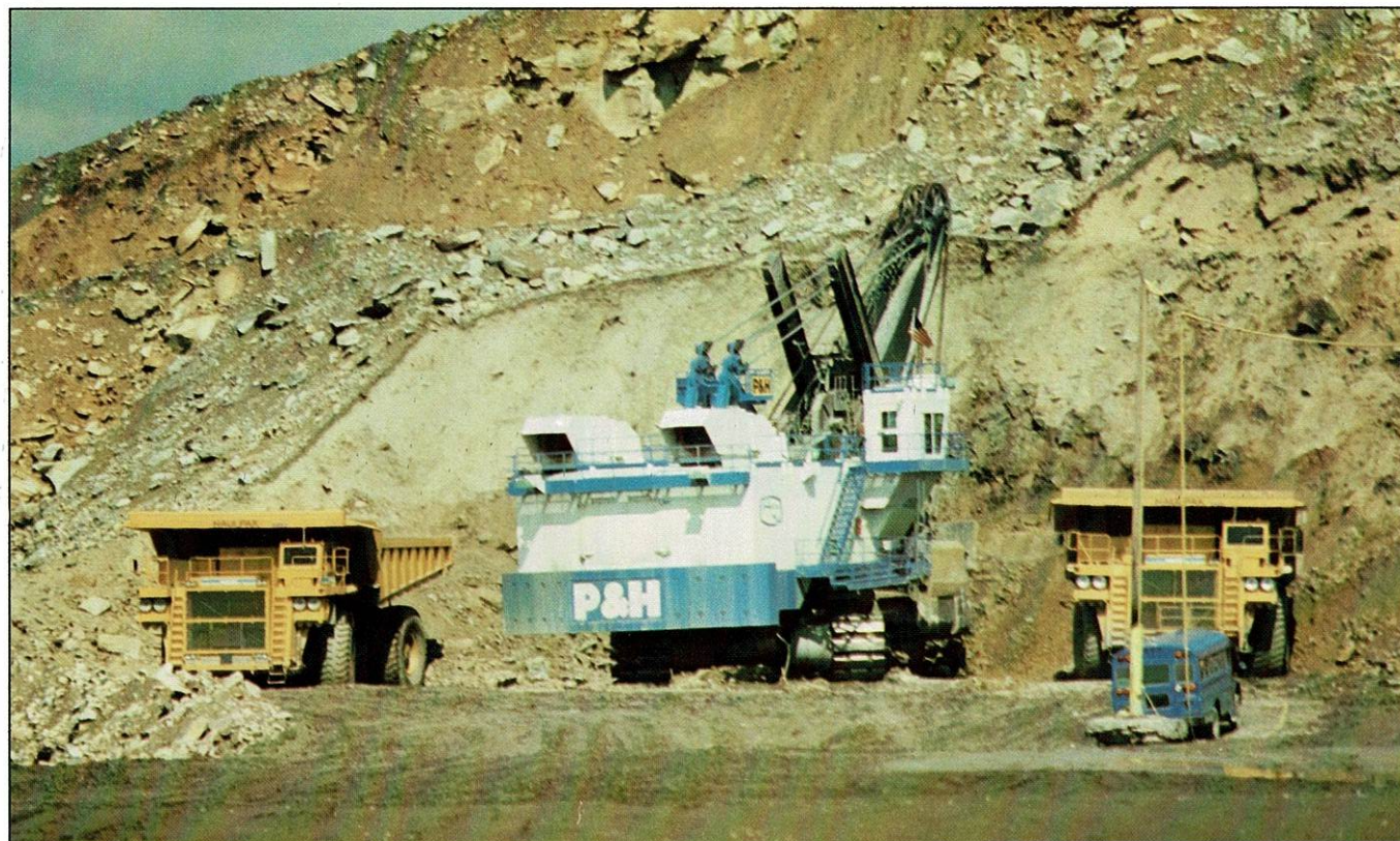
Wylo's 53 yard shovel works in conjunction with 240 ton rock trucks to uncover the Stockton and Coalburg seams.
