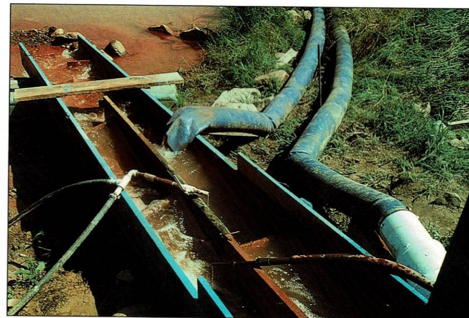
Figure 1. Sometimes several chemicals are necessary for suitable treatment of AMD. This site required the addition of an acid neutralizing reagent and also a flocculant to aid in precipitation of the metals.
