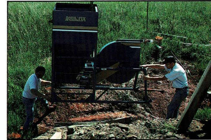
The Aquafix Machine is then situated over a fiberglass sluice carrying water beneath the unit.
