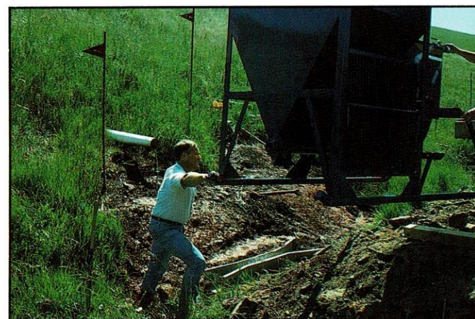
The machine weighs about 900 pounds and can be lifted into place by a tractor with a backhoe or a truck with a hydraulic lift.
