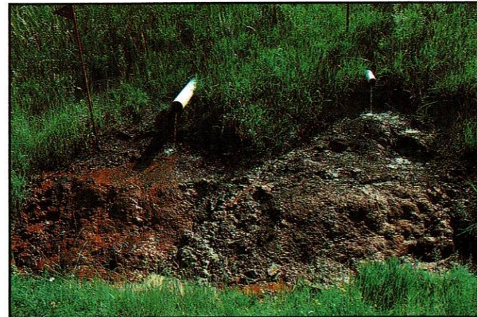
Seepage of acid mine drainage from a reclaimed backfill.
