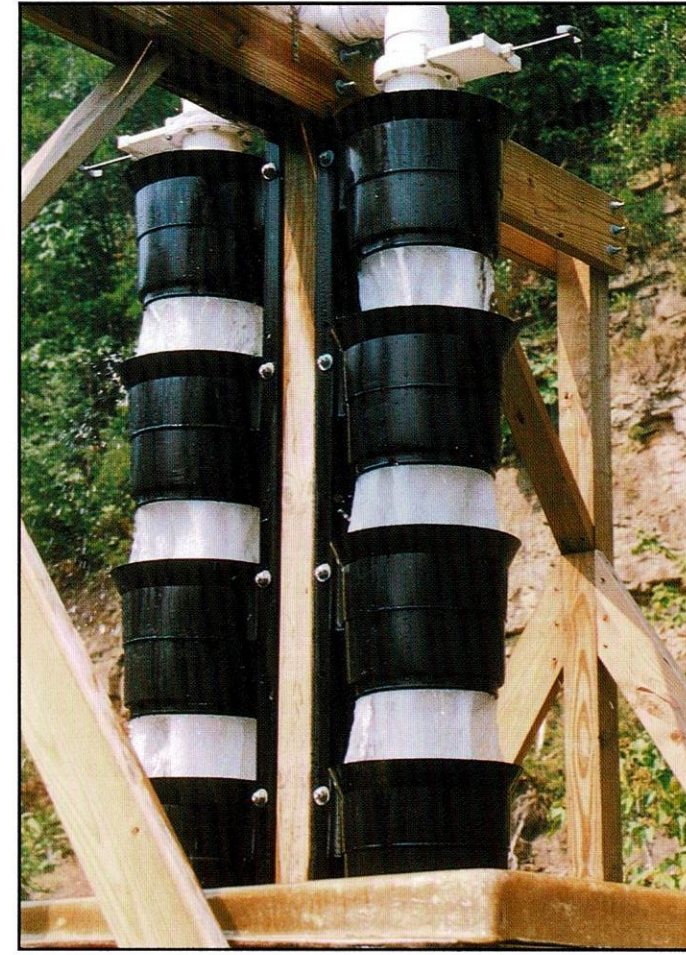
Water is oxygenated before flowing into the fish tanks by a simple mechanical means of exposing to fresh air.
