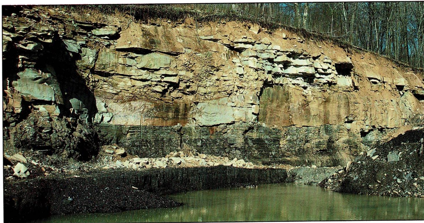
Figure 3. The alkaline material was placed on the pit floor after the Upper Freeport coal was removed. The pH of the water in the pit was maintained above 7.0.
