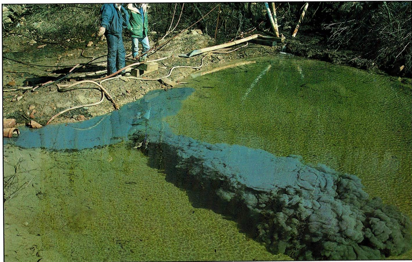
Figure 2 - Ammonia, when injected into acid mine drainage, reacts rapidly to raise pH and to neutralize acidity. Metals dissolved in the water will precipitate as the pH is raised.
