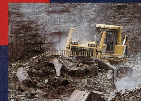
A D475A-2 Dozer pushing shot rock and overburden.
