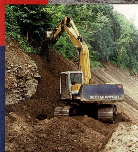
A PC200 LC-5 Excavator grading, loading and lifting on a reclamation project.
