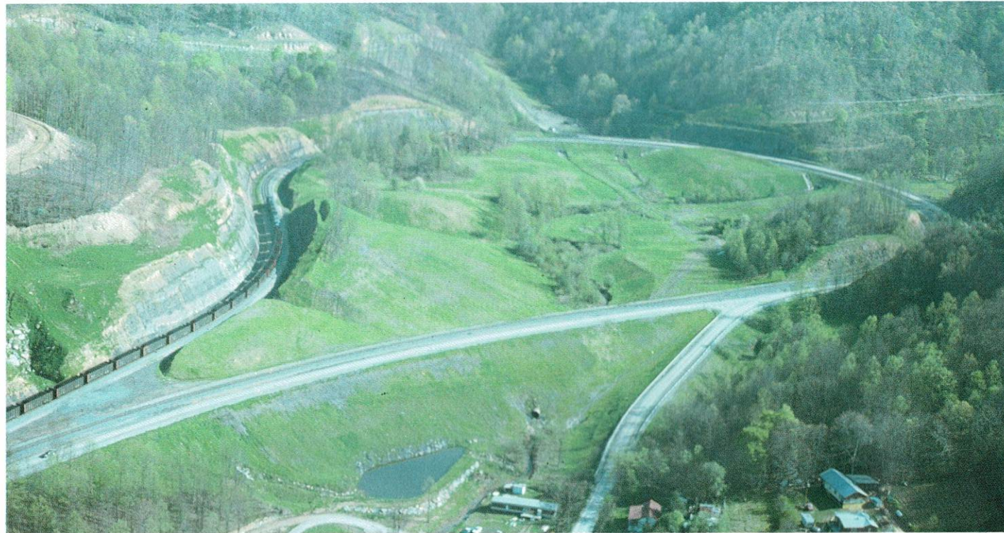
The railroad loop enables the coal train to move through the loadout facility efficiently.
