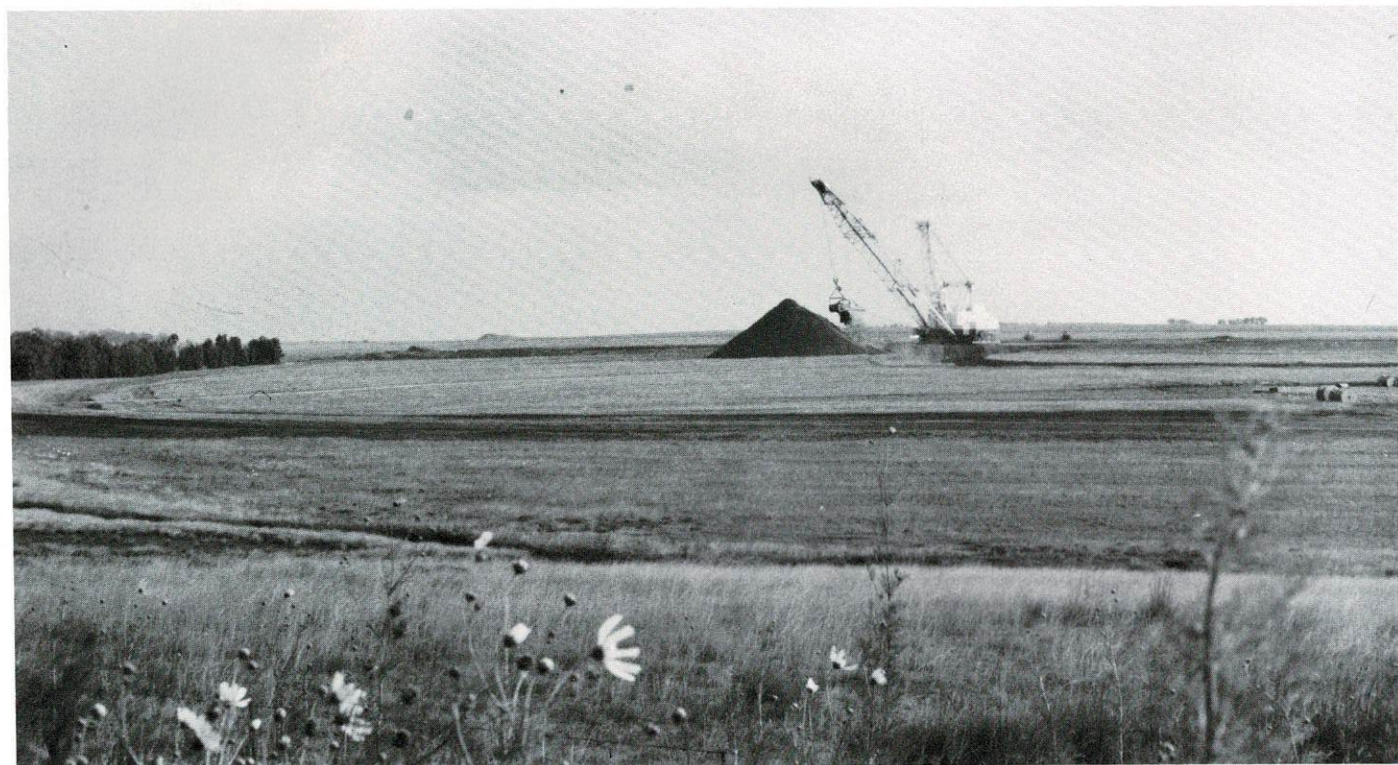
An American made dragline moves subsoil overburden in South African mining country.
