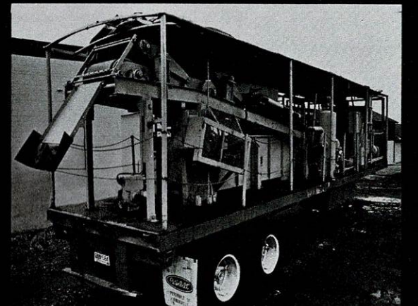
Fairchild's Belt Vacuum Filter Press Mobile Testing Unit Enables Us To Test Your Product On-Site. Through This On-Site Testing, We Can Determine The Unit To Best Serve Your Special Applications.
