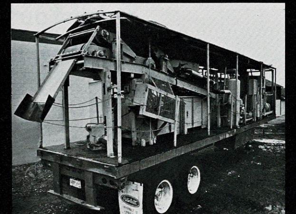
Fairchild's Belt Vacuum Filter Press Mobile Testing Unit Enables Us To Test Your Product On-Site. Through This On-Site Testing, We Can Determine The Unit To Best Serve Your Special Applications.
