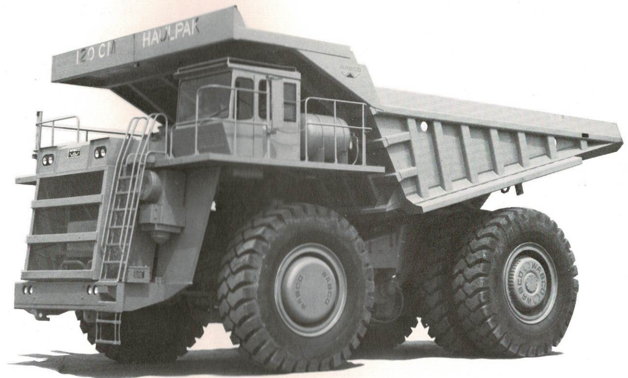
WABCO Haulpak 120 ton mechanical drive rock hauler.
