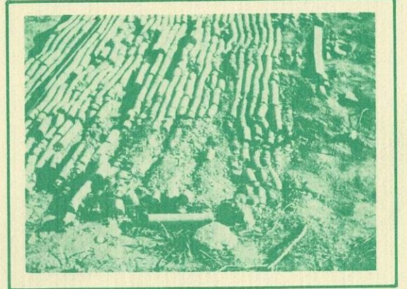
Above: Northern Preston County test core near Cuzzard, W. Va., which has been exposed to weather, showing differential weathering that occurs in blended minesoils. Core extends upward from Upper Freeport Coal.
