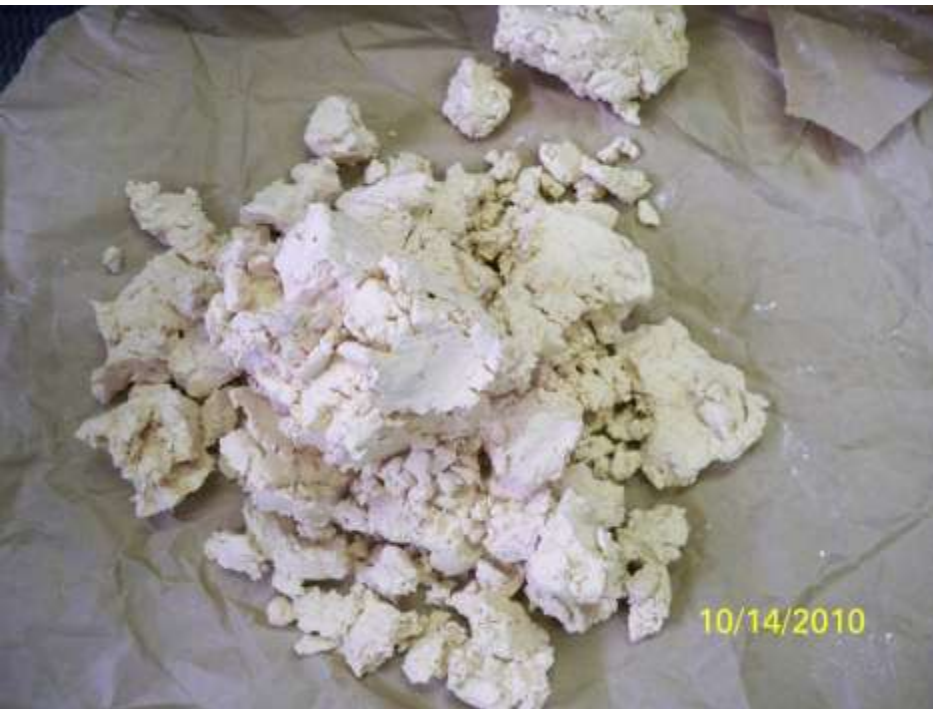
Dewatered Filter Cake
