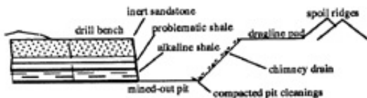
Figure 2 Configuration of Pit Prior to Blast Cast
