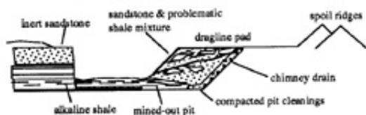
Figure 5 Configuration After Building Dragline Bench
